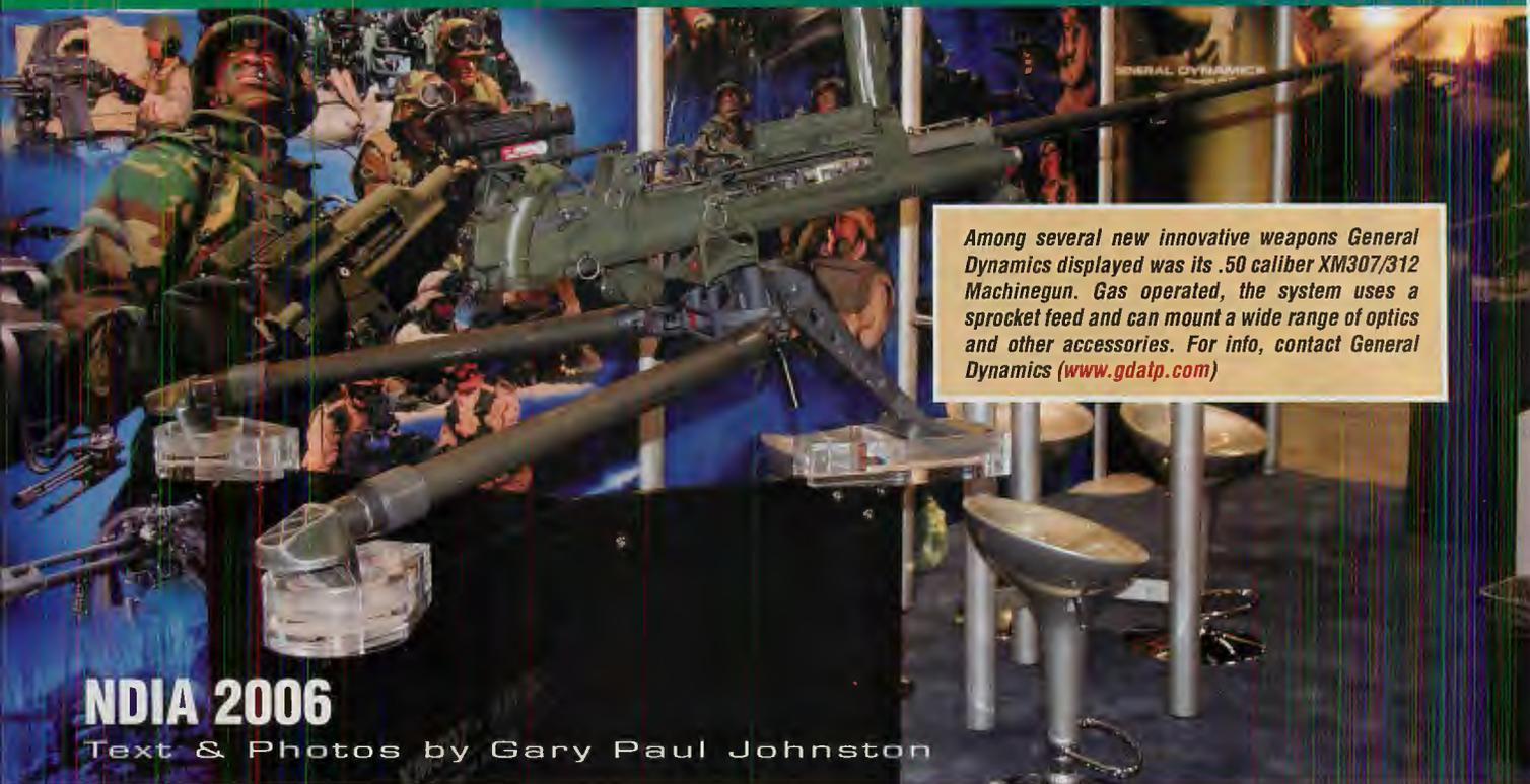
Among several new innovative weapons General Dynamics displayed was its .50 caliber XM307/312 Machinegun. Gas operated, the system uses a sprocket feed and can mount a wide range of optics and other accessories. For info, contact General Dynamics ([www.gdalp.com](http://www.gdalp.com))
